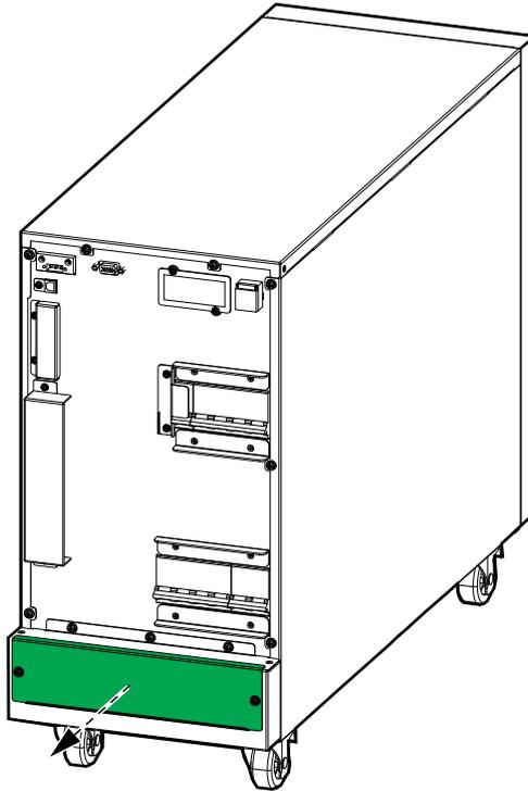
3. In dual mains systems, remove the single mains cable.
