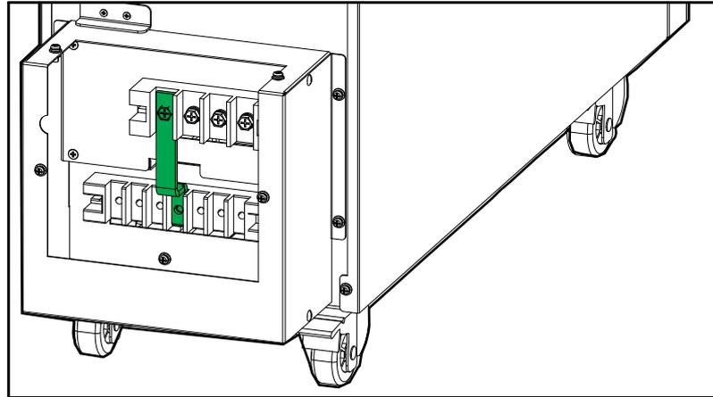
4. Route the power cables through the conduit box.
