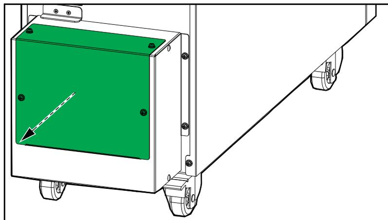
3. In dual mains systems, remove the single mains bracket.
