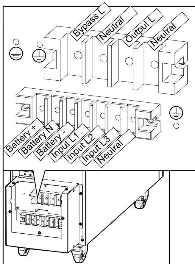
6. Connect the input, output, and bypass (if applicable) cables.
