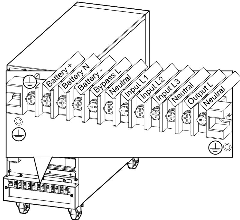
6. Connect the input, output, and bypass (if applicable) cables.
