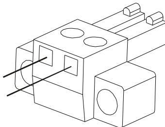
**The EPO interface is a Safety Extra Low Voltage (SELV) circuit. Connect it only to other SELV circuits. The EPO interface monitors circuits that have no determined voltage potential. Such closure circuits may be provided by a switch or relay properly isolated from the utility. To avoid damage to the UPS, do not connect the EPO interface to any circuit other than a unused circuit.**
