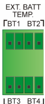
(Figure 4-10: External Battery Temperature Dry Contacts)
