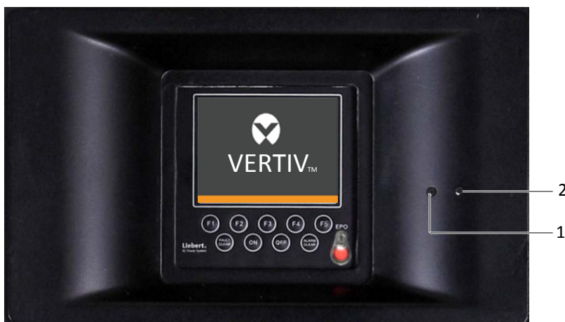
Figure 4-1 Operator control and display panel
