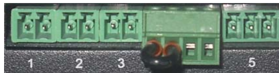
Figure 1-4 User dry contact and opto-coupled connectors
