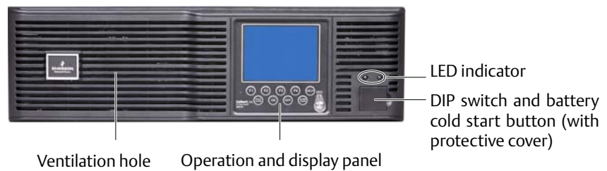
Figure 1-2 UPS module front panel
